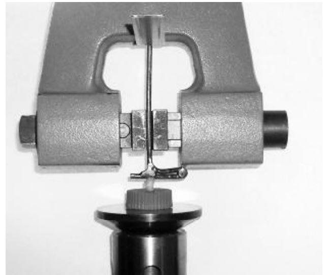
Fig. 3. Axial compressive loading: A – sample positioned in the Instron universal testing device, B – a steel metal cylinder 3.2 mm in diameter is used as plunger.
